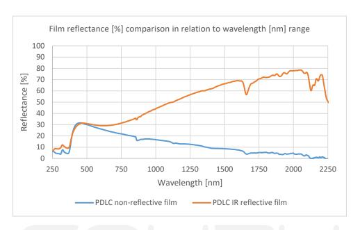
Above 1000 nm, IR PDLC films reflectance range increases and achieves 78%, at 2000 nm, while the regular PDLC films present 5%.
