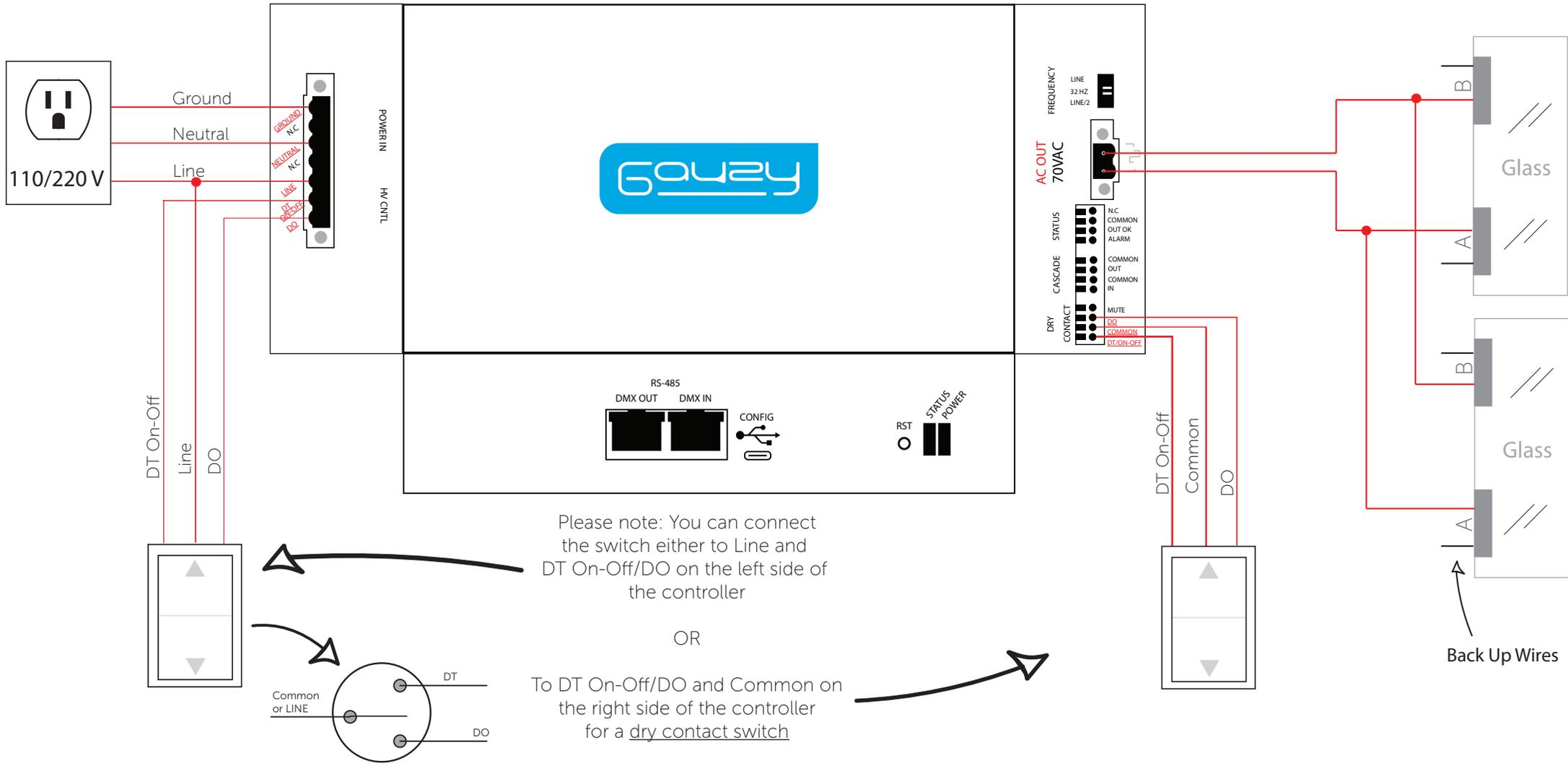
Please note: You can connect the switch either to Line and DT On-Off/DO on the left side of the controller
